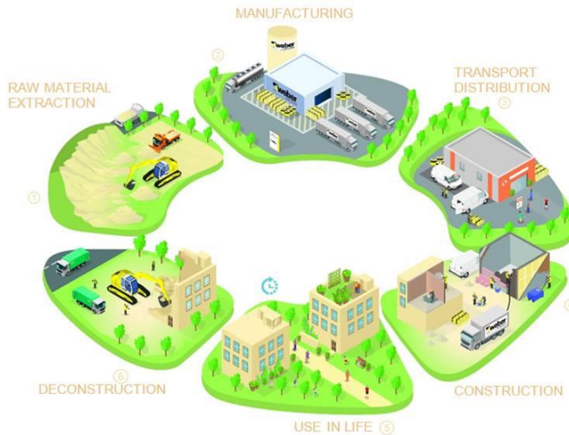
Figure 1: Cradle to grave analysis taking into account all stages of the Life Cycle product
